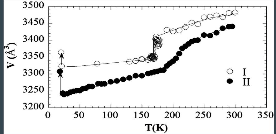
Temperature dependence of the unit cell volume around the spin transition.
