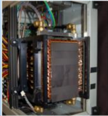
XPAD3 : 130 x 130 \mu\text{m}^2 pixels
